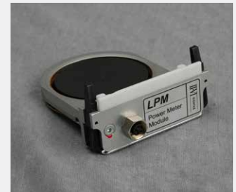
Laser power meter module (LPM) as insert in cover slide cartridge receptacle
